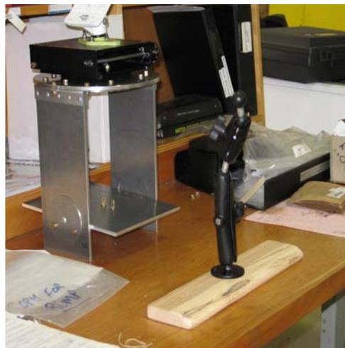
Figure 1. Foot-peg and operator-held video camera mounts built by OMNR-Muskoka staff.
